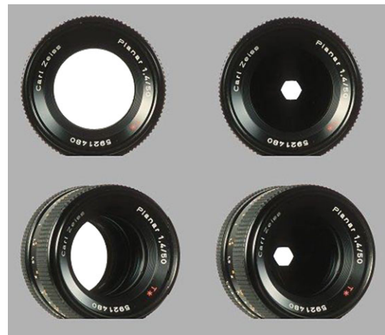
Fig. 3 The shape of the entrance pupil varies with both the aperture size and the angle of incidence. The white openings correspond to the clear aperture for light that reaches the image plane. (Image courtesy of Paul van Walree [33])
