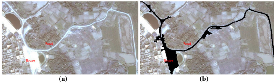
Fig. 1 Phenomenon of “different objects with the same spectrum.” (a) Initial image. (b) Mixed object consisting of a road and a house.
