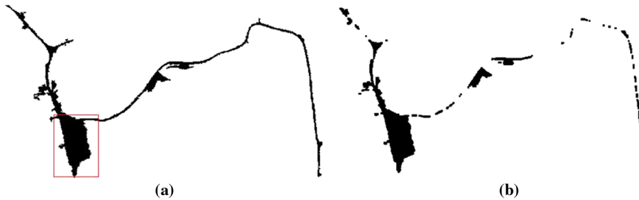
Fig. 2 (a) A mixed object. (b) The result of mathematic morphology with a disk construct element.
